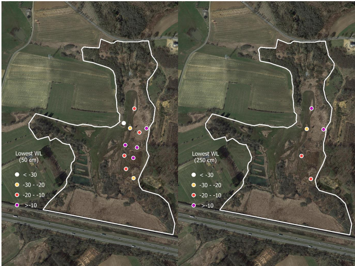
Figure 26. Lowest water level in shallow (left) and deeper (right) piezometers between april 2017 and april 2018
